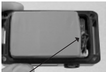
Pull on these wires carefully when removing the battery pack from the receiver.
