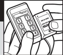
Before putting the collar on the dog, briefly touch the two red paper dots together (one on receiver, one on transmitter) to turn the collar on.
