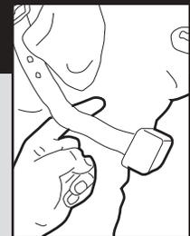
Proper Fit: The collar fit should be snug, yet loose enough to allow one finger to fit between the strap and the dog's neck. Fit is important because a loose collar may cause inconsistent performance. It's okay to trim any excess strap length.
