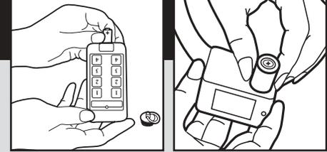
Transmitter: Insert 12v battery in the transmitter positive (+) side out. Replace metal cap.
