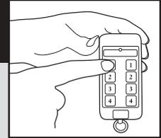
Press 1-LOW button in the DOG 1 column of the transmitter within 30 seconds of installing the receiver battery. The components now work together.
