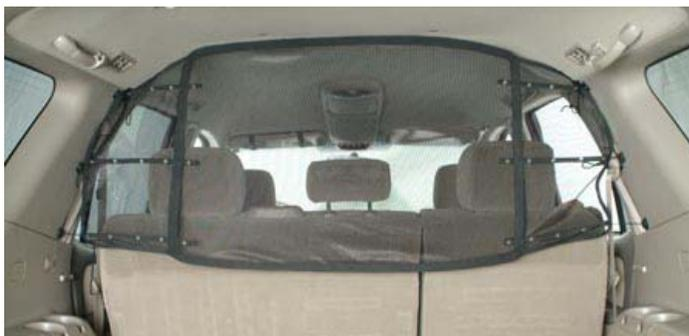
Step 1: The square fasteners must be attached to the plastic covers on the vertical columns which separate the windows - three fasteners per side - either behind the front seat or behind the back seat. **IT IS CRITICAL** that the square fasteners be attached to a super-clean surface (more on this later).
