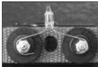
Test Light on Receiver Probes
