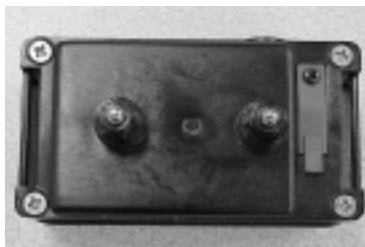
Remove these four (4) screws to replace the rechargeable battery pack.
